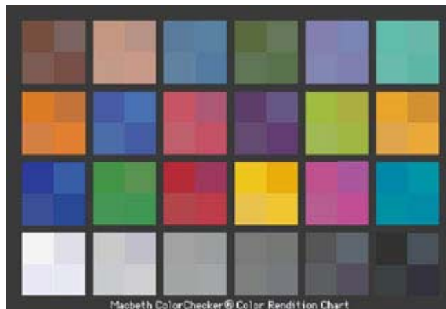
Figure 9: The Macbeth Color Checker is a standard color reference tool for photographers.
